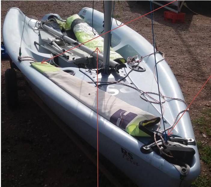
3. Place the **rolled mainsail in the hull**. Please do not fold it in half once rolled.
